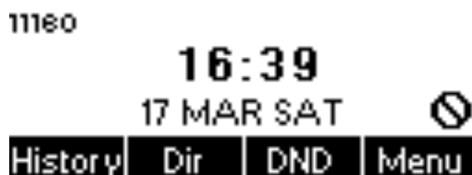
Figure 56 - DND Enabled on All Lines
